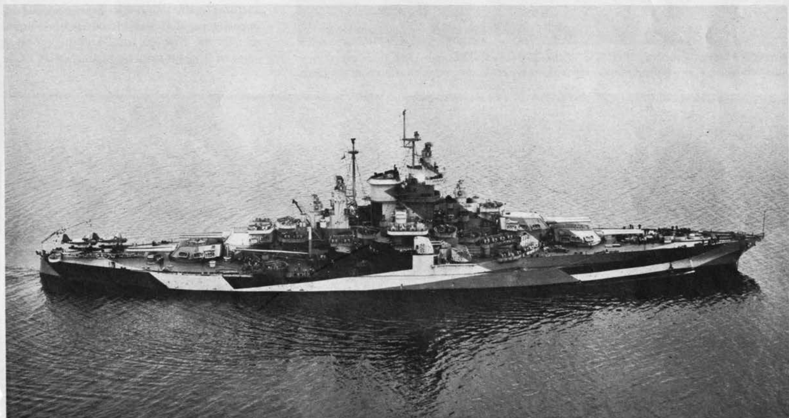
Enormous beam of the West Virginia leaves a broad parallel wake in a calm sea. Blisters which give her this bulk cut her speed somewhat but pay off in underwater protection.
